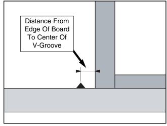
**Figure 22.** Groove cutting setup. (Side View)
